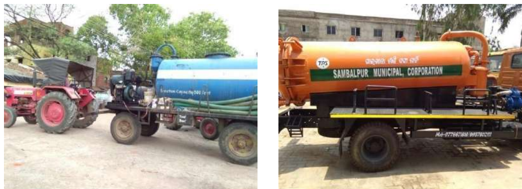
Figure 4-8: -Existing old vehicle (left) and new (right) cesspool emptying vehicles of SMC
